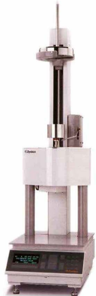
Melt Flow Rate Indexer
