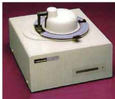
Oxidation Induction Time Tester
