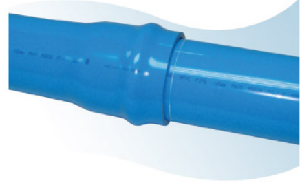
STEP 5 Insert the spigot end into the socket and apply steady pressure until the spigot slips through the rubber ring. Insert pipe until the reference line is just visible at the face of each socket.
