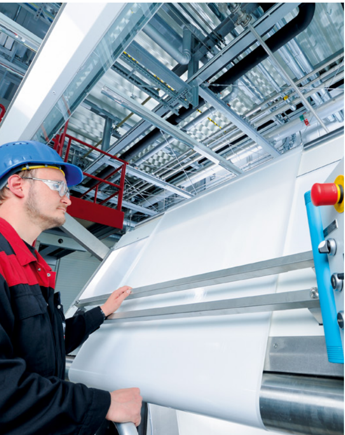
The membranes are based on a three-layer composite structure that is manufactured in several production stages. A single Lewabrane® RO element consists of a package with more than 20 layers. This is assembled into a spiral-wound element and then fixed.
