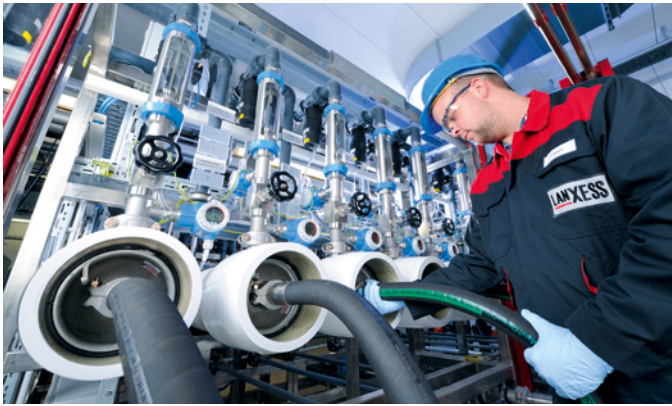
For quality assurance purposes each individual Lewabrane® product is checked in an element tester.
