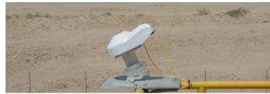
ISO 9060 Secondary Standard pyranometer No change of desiccant for 10 years Smart, more than just digital RS-485 Modbus® communication
