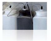
Continuous monitoring of the reagents through level probes. The powder DPD reagent to be diluted before use is an excellent solution for storing the product safely in any place.
