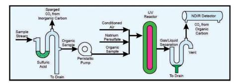
An on-board controller will process the data of the NDIR detector to calculate the concentration in mg/ or ppm.
