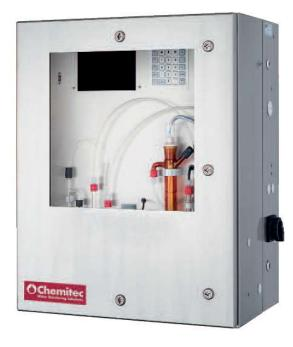
The **UVTOC-METER** is a continuous analyzer for the determination of total carbon (TC), total organic carbon (TOC) or dissolved organic carbon (DOC) according to the US-EPA Standard Method 5310C.
