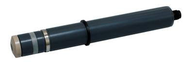
The chlorine sensor from the eCHEM sensors product range is an electrochemical sensor for measuring the chlorine concentration in water. This sensor detects free chlorine from inorganic chlorine products (chlorine gas, hypochlorite, etc.). The measuring method has a reduced pH dependency, so that pH fluctuations only have a limited impact on the measurement signal. pH value increases only lead to an approximately 10% reduction of the measuring signal per pH unit.
