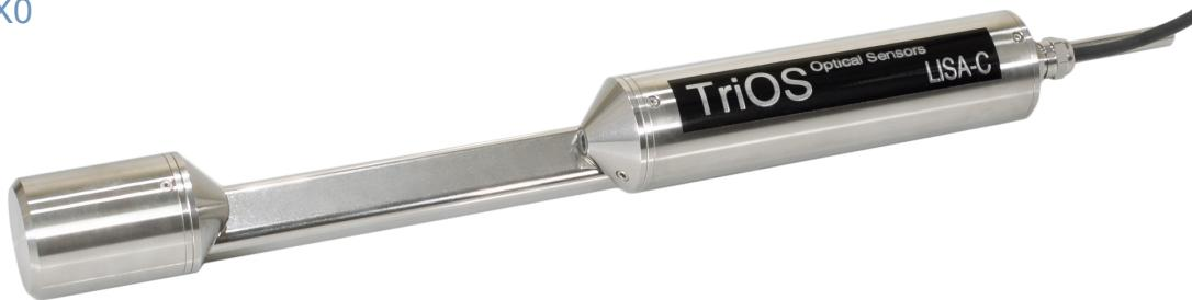
Colorimetry – LISA enables reliable low-cost colour measurements. The LISA color uses two different LEDs for long-term stable measurement of the SAC or color at different wavelengths. The second channel is used for turbidity/background correction. The cutting-edge device platform, used in all other TriOS photometers, enables optical path lengths of 50, 100, 150, and 250 mm, so that almost any application can be easily implemented.
