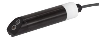
The TTurb is a digital sensor for optical turbidity measurement using the 90° IR scattered light method. Depending on the sensor design it can be used in pure water up to 100 FNU as well as in raw water, waste water and process water up to 1000 FNU. TTurb is available with different cable lengths (10 m or 2 m) as well as in different versions.
