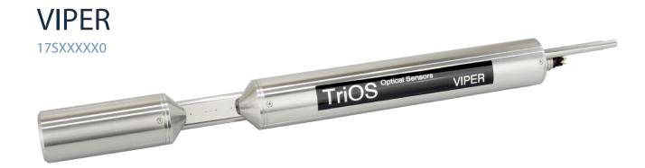
VIPER measures hyperspectral attenuation and transmission coefficients in the wavelength range of 360 nm and 750 nm, enabling detailed determination of multiple parameters at the same time. The light source is provided by 5 selected, energy-saving LEDs that Warranty a long service life and stable measurement data. VIPER can be used in different media as it is available in multiple path lengths, both in stainless steel or titanium housing.
