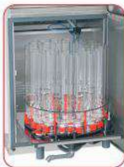
Distributor with glass bottles, placed on a telescopic drawer
