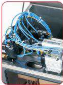
Fold-out plate with Ex valves and diaphragm vacuum Ex pump
