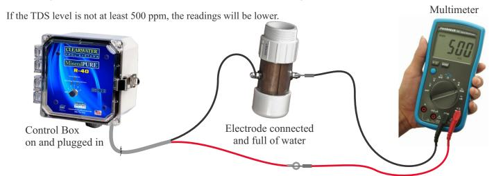
The electrode chamber must be full of water with the filtering system on for this to give you an accurate readout.
