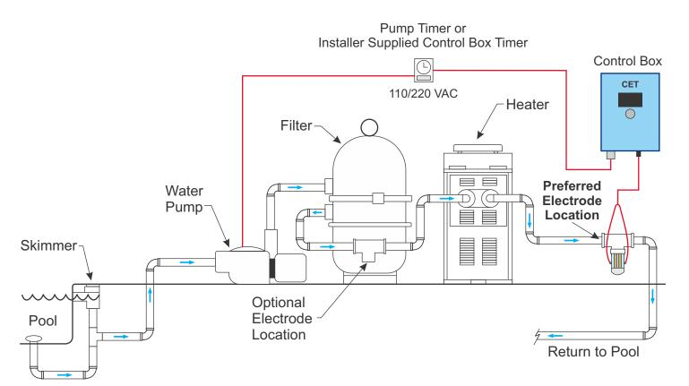
The <u>MineralPURE R-40</u> should be installed at the pool's pump and filter area. The preferable location to mount the electrode chamber(s) is <u>after</u> the pool's pump and filter, but it can be installed before the pool's pump and filter if needed. The electrode chamber(s) will need to be within 10 feet of the control box for an electrical connection. The control box will need to be within 7 feet of an electrical source.
