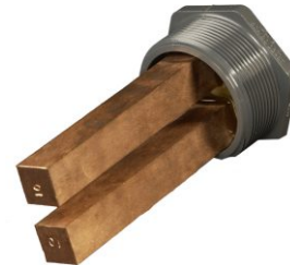
7" long 90% copper, 10% silver electrode, 3" sch 80 (CLE-20)
