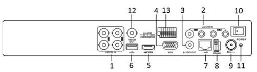
\*: The rear panel of DS-7208/7216HUHI-K2/P provides 8/16 video input interfaces.
