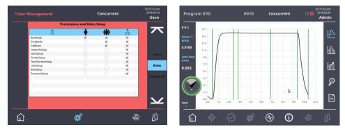
The reimagined touchscreen provides access to a wide range of data. From statistics like pass, fail, minimum, maximum, and standard deviations, to historical graphs and charts, the Sprint<sup>mD</sup> provides a deep level of information, making it easy to monitor the process.
