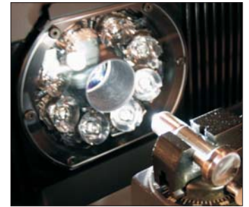
Motorized CC-14 shown with optional Quadra-Chek QC-300 DRO and TruLight Ringlight.
