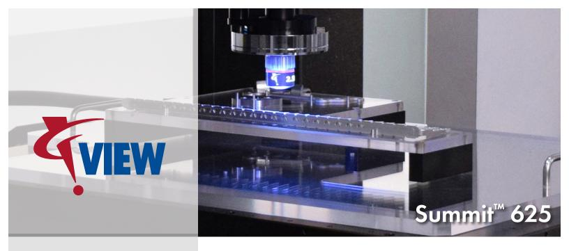
VIEW Summit 625 delivers high accuracy and high measuring speeds for near-line process monitoring and quality assurance applications. XY stage velocities of up to 400 mm/sec (with optional linear motor drive) ensure very high productivity on the factory floor.
