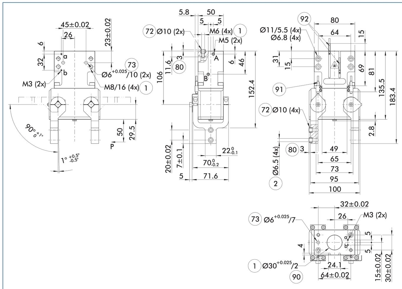
The drawing shows the gripper in the basic version with closed jaws, without dimensional consideration of the options described below.
