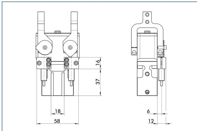
The attachment kit consists of brackets and the appropriate fastening materials. The proximity switches must be ordered separately.
