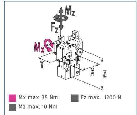
① The indicated torques and forces are static values, apply for each base jaw, and may occur simultaneously.
