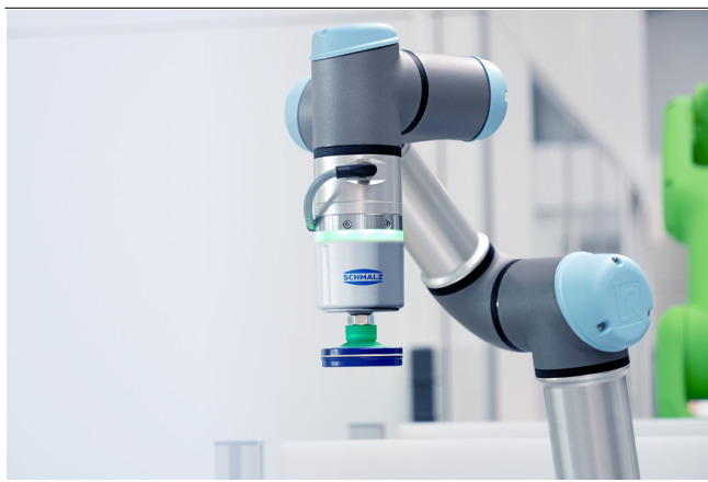
Electric vacuum generator ECBPMi for handling cans
