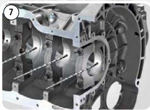
7 Bohren Kurbelwellenschmierung Boring of lubrication holes for crankshaft
