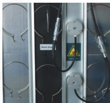
Four sensors monitor UV irradiance
