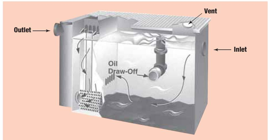
Note the course of water travel in cut-open view. The arrows designate the course from the inlet through the first separating screen, upward and through the second separating screen, downward through the filter and flow regulator screen to the outlet, and upward to the drainage line. There is no straight in-and-out travel from the inlet to the outlet of the interceptor.
