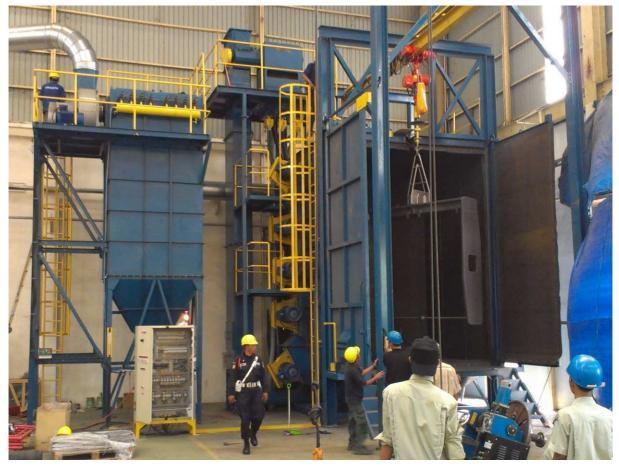
Above picture showing Model MR1011 machine with a capacity of 3 tons rotating hanger & work size of 3x3mW x 4mH. Five blast wheel units are installed with this machine.
