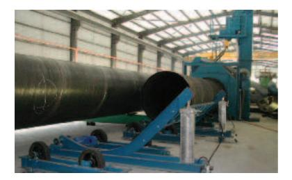
Completed system fully installed and commissioned for running at site of a pipe maker plant. The main products are cement lined water pipes.
