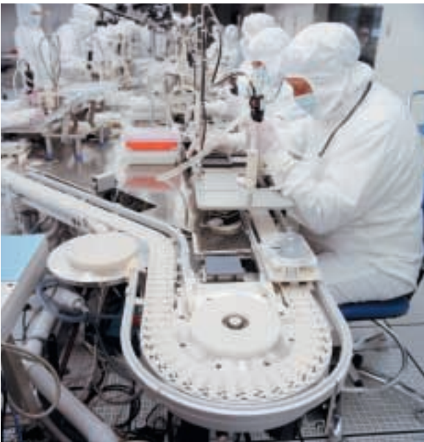
DELRIN® low wear low friction grades in conveyor chains allow for a longer lifetime of chains and wear strips, smooth sliding of the conveyed goods, silent (squeak free) motion and lubrication free operations.
