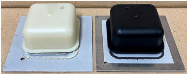
Cohesive failure after burst testing a cube (15 bar on left, 10 bar on right) shows failure in the weld joint and not the interface between metal and ZytelBond™.
