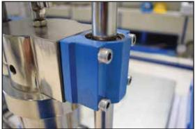
Equipped with bearing for smoother compaction drop
