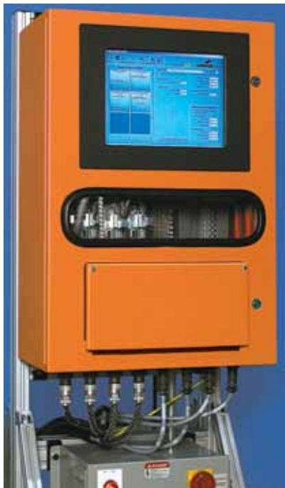
The Mid-Six controller is a wall mount design capable of handling up to six spindles and has all of the features as our larger panels.
