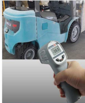
The whole vehicle can be operated alternately in 20°C cold storage for 6 hours and parked in the cold storage for 12 hours without any failure and can continue to work.
