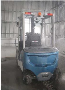
IPX4 waterproof: the vehicle is powered on to simulate a 15min short-time 5000L rainstorm test, and the vehicle can continue to run without failures.
