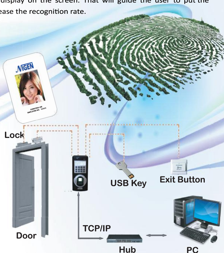
Door Access Connection Diagram
