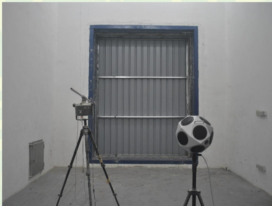
Photo 2: Test setup for testing of sample in Source Room
