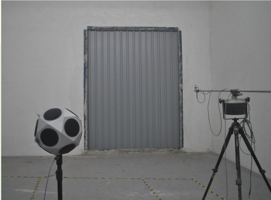
Photo 1: Test setup for testing of sample in Receiving Room
