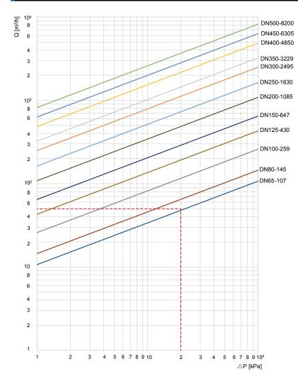
As shown in the left, it is the flow chart of Static balancing valve DN65-DN500 when the valve is full open. For example:
