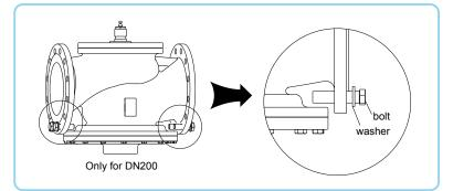
3. Valve and actuator can be assembled easily.
