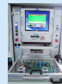
Automatic PCBA ATE test platform
