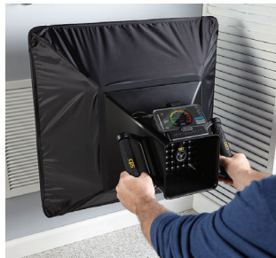
Included expansion hood captures airflow from grilles up to 24" x 24" (.6 x .6 m)
