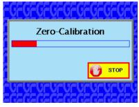
Zero calibration is used to calibrate the hardware. It is **not** calibration of the substances in the beer. This is performed with the B calibration. If you would like to check the zero calibration process, please carry out a control measurement with distilled water. For this control measurement profile 0 must be used. Profile 0 cannot be calibrated and is therefore suitable for this control measurement.
