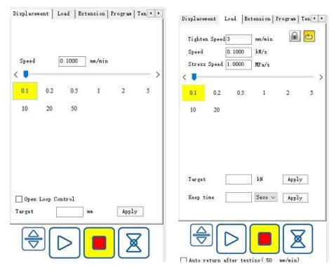
(3) Automatic program-controlled intelligent expert system. Up to 50 steps can be automatically programmed.
