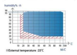
Can support the humidity from 20% to 98% in the temperature range of +10 to 85, to maximize the simulation of the atmospheric environment, can design a variety of tests.
