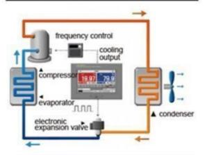
Through the controller output signal, control the frequency converter and electronic expansion valve, accurately adjust the refrigerant flow, in order to achieve energy saving effect, and the cooling system will more stable. (Frequency control is optional)
