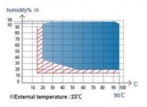
Can support the humidity from 20% to 98% in the temperature range of +10 to 85, to maximize the simulation of the atmospheric environment, can design a variety of tests.
