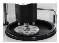
quickly replaced; multi-sample holder and pneumatic single-point loading and other functions.
