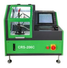
CRS-206C common rail injector tester it can test common rail injector of BOSCH, SIEMENS, DELPHI and DENSO as well as piezo injector. BIP functin, QR code function available. Windows operating system, Linux operating system both available.
