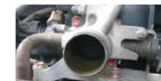
BEFORE (Throttle body condition after 60,000 km)
