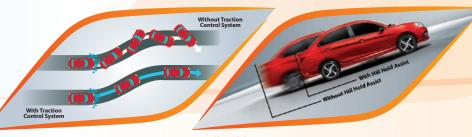
Electronic Stability Control and Traction Control System Hill Hold Assist
