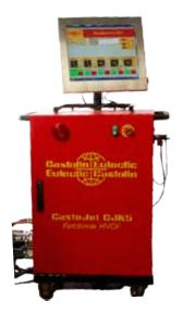
The CastoJet<sup>®</sup> Kerosene 5 - CJK5 - is the latest Castolin Eutectic development of kerosene fuelled high pressure HVOF (High-Velocity Oxy-Fuel) systems. Using mass flow control for repeatable coating quality. The system produces the densest metallic and carbide coatings of all. The coatings can be compressively stressed, allowing thick layers to be applied without fear of spalling.
