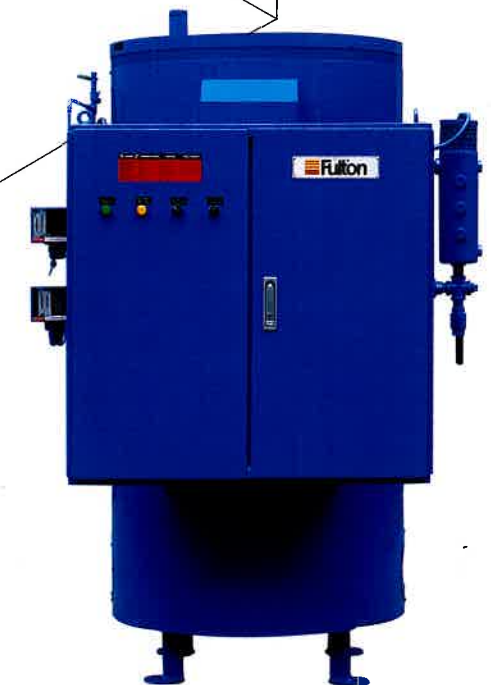
300 to 2000 kW (30 to 200BHP) Elements are vertically mounted. These boilers have an externally mounted water bottle assembly housing the low water cut-off probe, pump on probe and pump off probe. The second (auxiliary) low water cut off probe is mounted in the top of the boiler.
