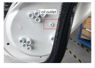
Location of oil outlet and inlet of 3rd-axis:
