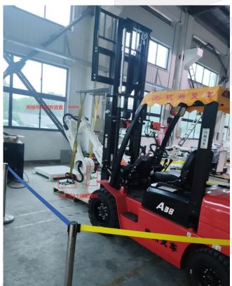
Note: Operators who assist on the side must wear protective shoes and helmets. During the entire lifting process, the assisting personnel must not place their limbs under the robot arm to avoid injury.
