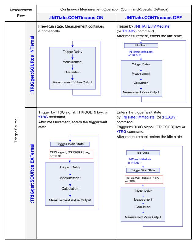
If the :INITiate:CONTinuous OFF has been set, when operation is returned to the Local state or the power is turned off and then back on, the :INITiate:CONTinuous ON state occurs.
