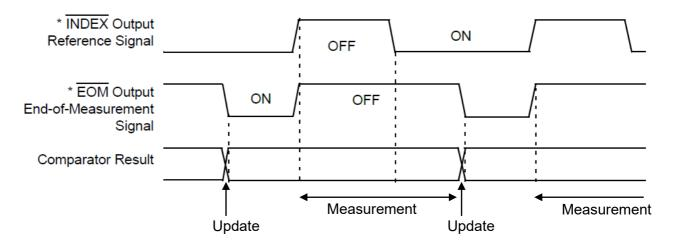
Holds the previous comparator result during measurement. The Comparator result is updated when the measurement is completed.
