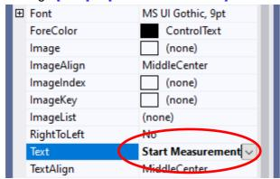
4. The [Start Measurement] is placed on the form.
