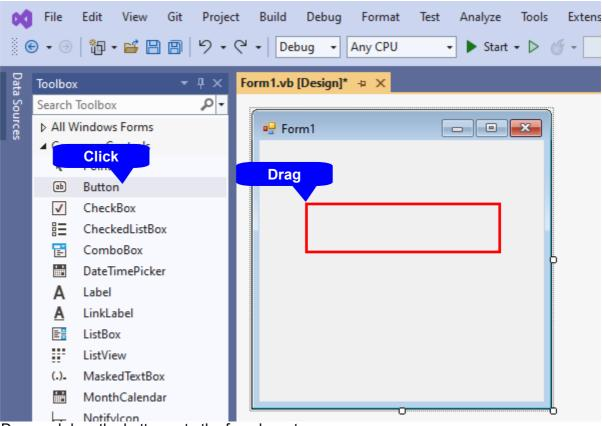
2. Drag and drop the button onto the form layout screen.
