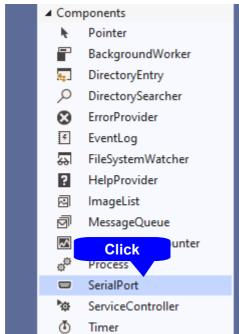
2. Drag and drop the [SerialPort] component onto the form layout screen.
