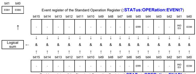
Enable register of the Standard Operation Register (:STATus:OPERation:ENABle)
