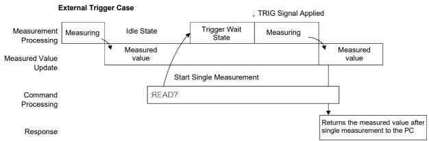
Use this method to measure (and export) synchronously with the controller (PC, PLC) or external trigger signal. Measurement time can be minimized.
