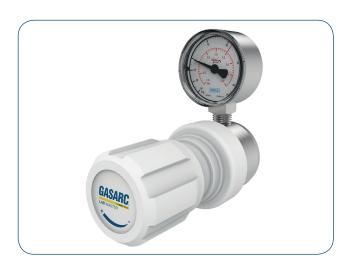
The Lab Master LGP510 Series single stage diaphragm outlet point regulators are designed for secondary pressure gas control of high purity Acetylene gas up to grade 5.0 purity (99.999%), on gas distribution systems.
