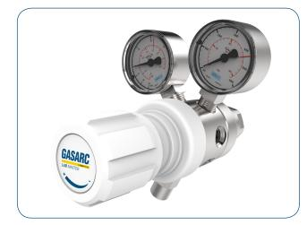
The Lab Master LGT510 Series two stage diaphragm cylinder regulators are designed for primary pressure gas control of high purity Acetylene gas up to grade 5.0 purity (99.999%), on applications where constant delivery pressure is required as cylinder pressure decreases.
