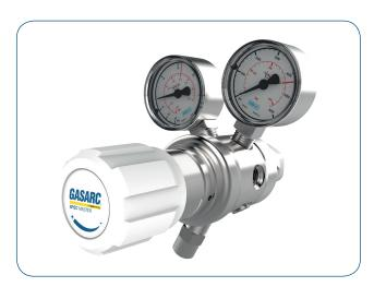
The Spec Master HPT600 Series two stage diaphragm cylinder regulators are designed for primary pressure gas control of non-corrosive or toxic, high purity gases up to grade 6.0 purity (99.9999%), on applications where constant delivery pressure is required as the cylinder pressure decreases.
